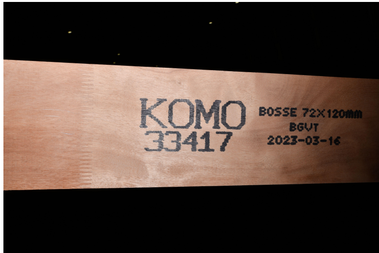
Komo certified finger-jointed glulam - Interholco production (© Alain Mazeau)
